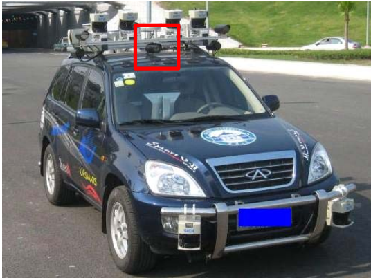
Fig.8. SmartV, which is an intelligent vehicle developed by Wuhan University. It has CCD cameras, lasers, GPS and IMU, etc. Camera labeled is used to acquire road images.
