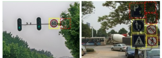
Fig.9 Failure cases of Traffic sign detection. Detected and missing traffic signs are marked by yellow bounding box and red bounding box.
