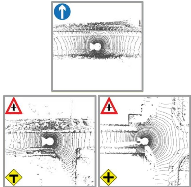
Fig. 1. The goal of intersection recognition is classifying situations ahead of a vehicle as intersection and road segment, and in addition, making a distinction between T-shaped and +-shaped intersections.
