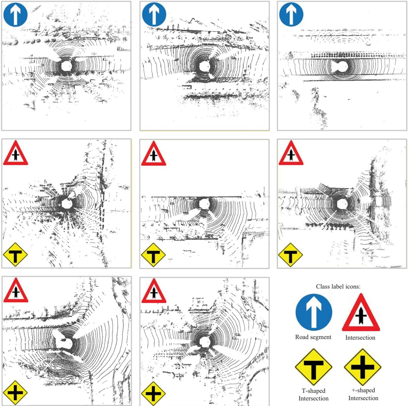
Fig. 7. Examples of successful classification. The first row are examples of road segments; the second row are examples of *T*-shaped intersections; the last row are examples of "+"-shaped intersections.
