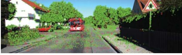
Fig. 5. This figure displays the outliers (red) and inliers (green). The outliers are mainly located on the moving bus. For other mismatched outliers, we use the SPS method to reduce the noises during capturing the final result.
